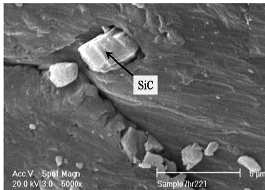
Fig. 5. SiC powder embedded within an aluminum matrix after 5 h of milling.
