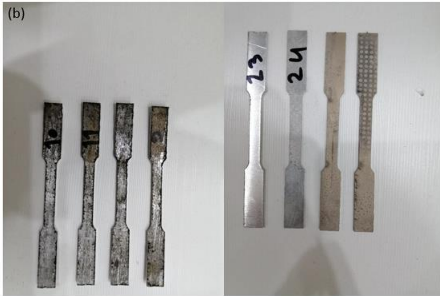
Fig.1. (a) Tensile test specimen design according to ASTM-E8M, (b) prepared tensile test sample
