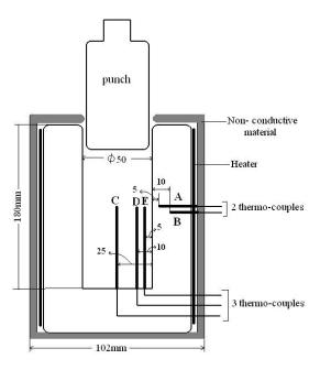
Fig. 5. Mold assembly and thermocouples position.
