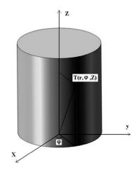
Fig. 2. Cylindrical coordinate system.
