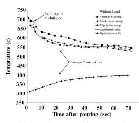
Fig. 8. experimental measured temperatures of solidification of A356 Al with time (Atmospheric).
