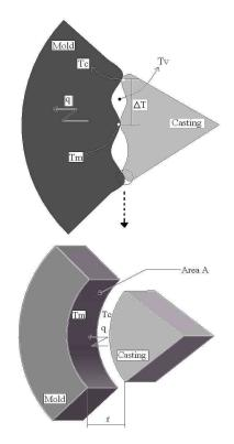
Fig.1. Representation of heat flow across permanent mold–casting interface.
